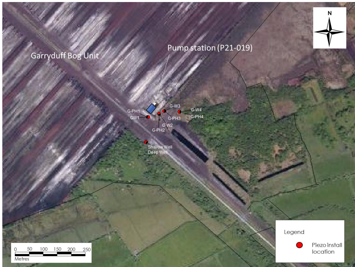
Figure E: Garryduff - piezometer install location map
